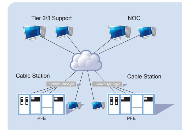
An unlimited number of operator positions can be implemented using any Windows® PC as a workstation. Station, NOC and support staff can all have access, with no additional capital investment in hardware.
